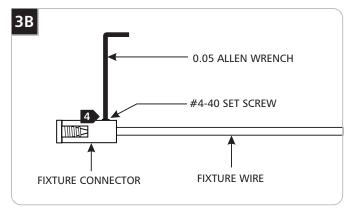
Tighten the #4-40 setscrew with the 0.05 Allen wrench.
