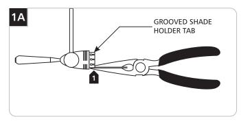
If the Bell shade fits tight onto the fixture, then carefully bend the grooved shade holder tabs in slightly with the needlenose pliers. If it fits loose, then carefully bend the grooved shade holder tabs out slightly with the needlenose pliers.
