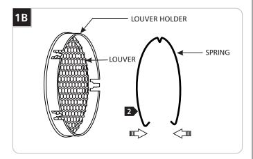
Place the louver in front of the louver holder. Squeeze the spring ends together and place it in front of the louver holder.
