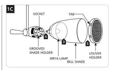
Use MAX 35 Watt, MR16 Front Cover Halogen Lamp with Bell shade.
