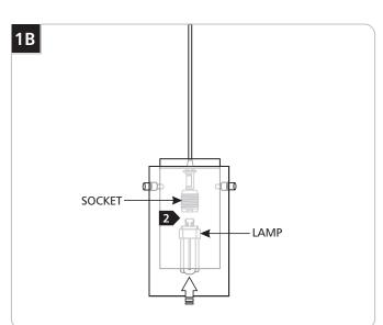
Use MAX 18 Watt GX24Q-2 Base Triple Tube Compact Fluorescent Lamp.
