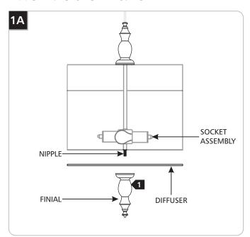
1 Place the diffuser onto the nipple and secure it to the socket assembly by tightening the finial.
