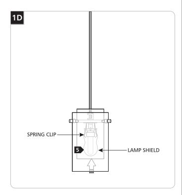
5 Push the lamp shields onto the spring clips.
