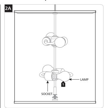
Use **MAX** 120 Volt, **150** Watt A21 (medium) base lamp with each socket.
