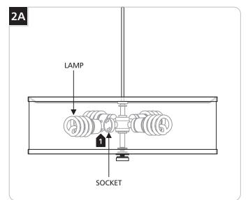
Use **MAX** 120 Volt, **18** Watt Type GU24 Base Self Ballasted Spiral Compact Fluorescent Lamps.
