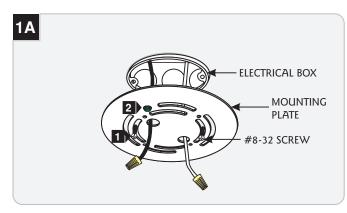
Install the mounting plate to the electrical box with the two #8-32 screws provided.
