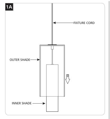
1 Feed the fixture cord through the outer shade and gently slide the outer shade onto the inner shade.
