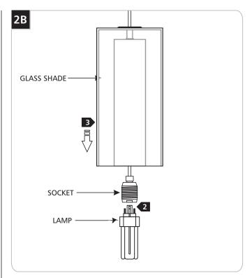
Use MAX 32 Watt GX24Q-3 Base Triple Tube Compact Fluorescent Lamp.
