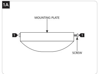
1 Separate the mounting plate from the canopy by removing the two screws.
