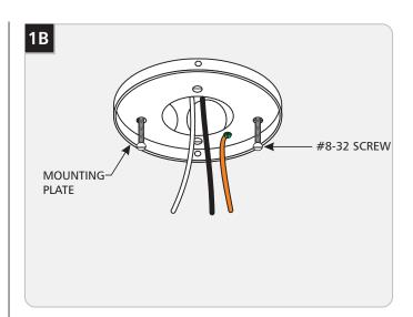
2 Secure the mounting plate to the electrical box with the two #8-32 screws provided.
