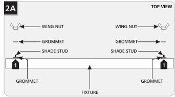
Remove two wing nuts and two grommets from the shade studs on the front of the fixture base. Ensure that a grommet remains on each shade stud.
