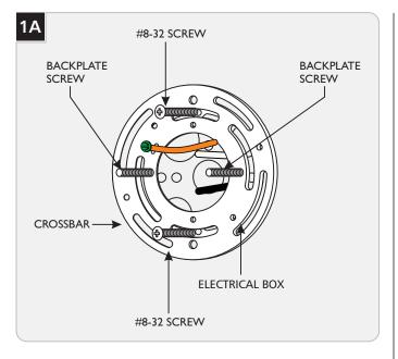
1 Snugly mount the crossbar to the electrical box with the two #8-32 screws provided.
