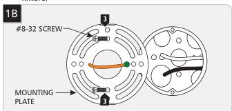
Secure the mounting plate to the electrical box with the provided #8-32 screws.
