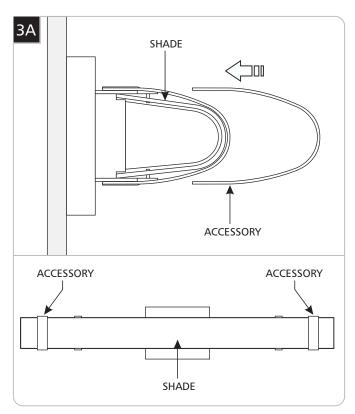
Slide the accessories onto the glass, until it snaps into place, at the desired location.
