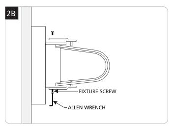
2 Secure the shade by installing the brackets and tightening the bracket screws with the provided Allen wrench.
