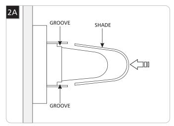
1 Install the shade into the grooves in the fixture base and hold it in place.
