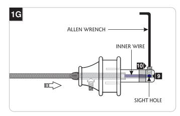
Look into the sight hole on the top of the connector to make sure that the inner wire is contacting the end of the connector.
