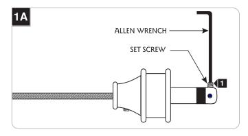
Back out (do not remove) the set screw on the tip of the connector with the provided Allen wrench.
