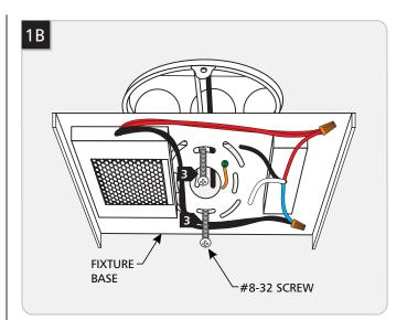
Secure the fixture base to the electrical box with the two #8-32 screws provided.
