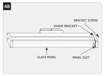
Install the glass panel into the panel slot on the installed shade bracket, install the other shade bracket while ensuring that the glass panel is in the panel slot, and secure them in place by installing and tightening the other bracket screw.
