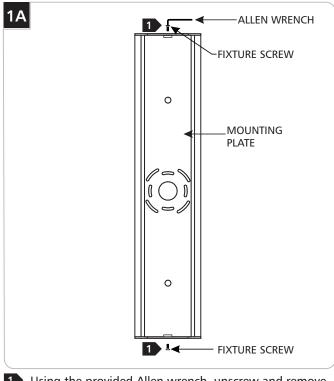
1 Using the provided Allen wrench, unscrew and remove the two fixture screws located at the top and bottom of the fixture
