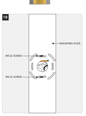
3 Attach the mounting plate to the electrical box using the two #8-32 screws provided.
