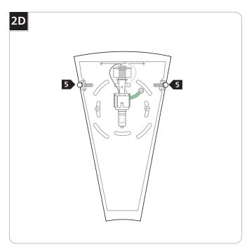
Firmly push the glass against the wall and finish tightening the ball screws.
