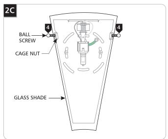
4 Slightly screw (**Do Not Tighten**) the ball screws through the glass shade holes into the cage nut holes so that the glass shade is held in place.
