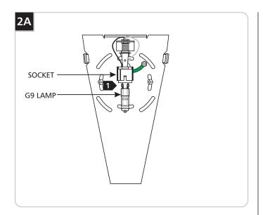
**NOTE:** The G9 lamp has an integral glass envelope and is thus safe to be used without a lamp shield.
