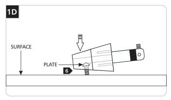
6 Tap the conical connector on a hard surface with the set screw facing down, so the plate inside drops into place.
