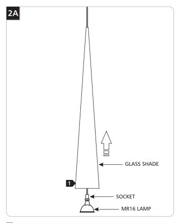
1 Move the fixture glass shade up to expose the socket.
