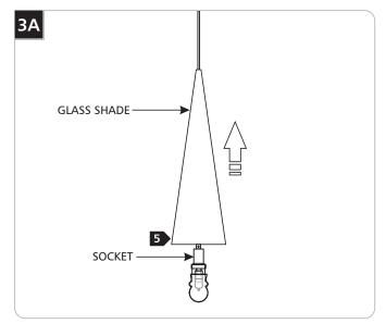
**5** Lift the glass shade up to expose the socket.
