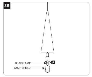
6 Remove the lamp shield and the old lamp.
