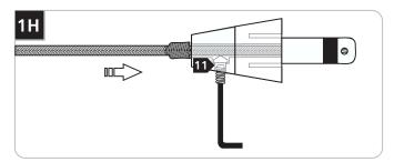
11 Firmly tighten the set screw on the conical connector.
