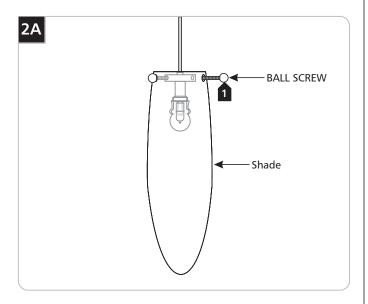
To remove the shade, hold the shade with one hand and unscrew the three ball screws with the other hand.
