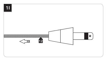
12 Pull the coaxial cable toward the fixture to smooth the wrinkles.
