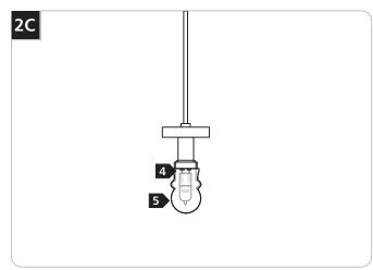
For incandescent versions, use MAX 50 Watt Bi-Pin Halogen Lamp.
