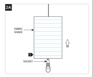
1 Lift the fabric shade up to expose the socket.
