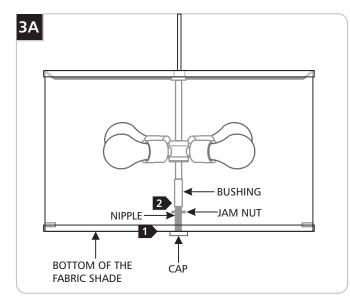
Loosen the knurled nut and adjust the nipple height so the back of the cap is level with bottom of the shade.
