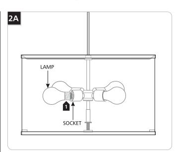
Use **MAX** 120 Volt, **150** Watt A21 (medium) base lamp with each socket.
