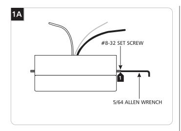
Back out (DO NOT REMOVE) the two #8-32 set screws for 1/4" with the 5/64 Allen wrench.
