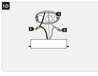
4 In accordance with local electrical codes, ground the fixture bare wire.
