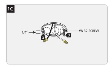
3 Thread (NOT COMPLETELY) the two #8-32 screws into the electrical box holes leaving 1/4" of them exposed.
