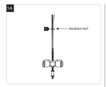
1 Unscrew and remove the knurled nut from the socket assembly.
