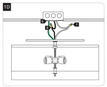
NOTE: Use the provided universal round crossbar when the canopy holes do not line up with the electrical box holes.
