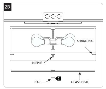
2 Place the glass disk onto the nipple and secure it against the shade pegs with the cap.
