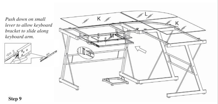
Place rubber suction cups (E) on keyboard tray frame (Q) and place keyboard tray glass (M) on top of the rubber suction cups. Now take the keyboard tray and slide it into the keyboard tray arm (I). Find desk glass (K) and (L). Place the glass on top of the desk frame according to the above illustration.
