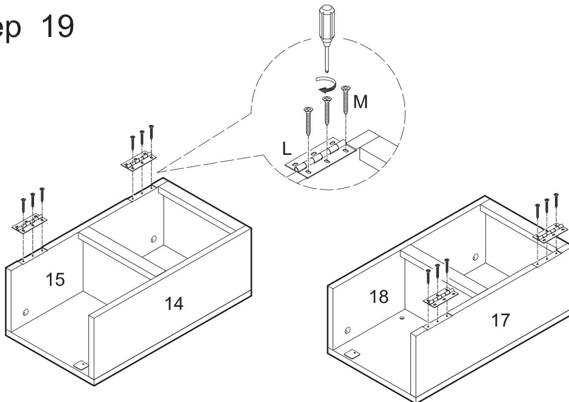
Attach door hinges (L) to the door assemblies from Steps 8 and 9 using large screws (M).
