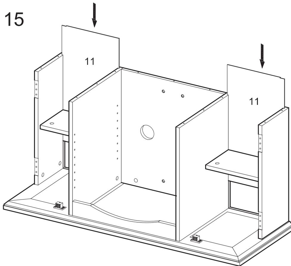
Carefully slide back panels (11) into place along the grooves at the back of the stand assembly.
