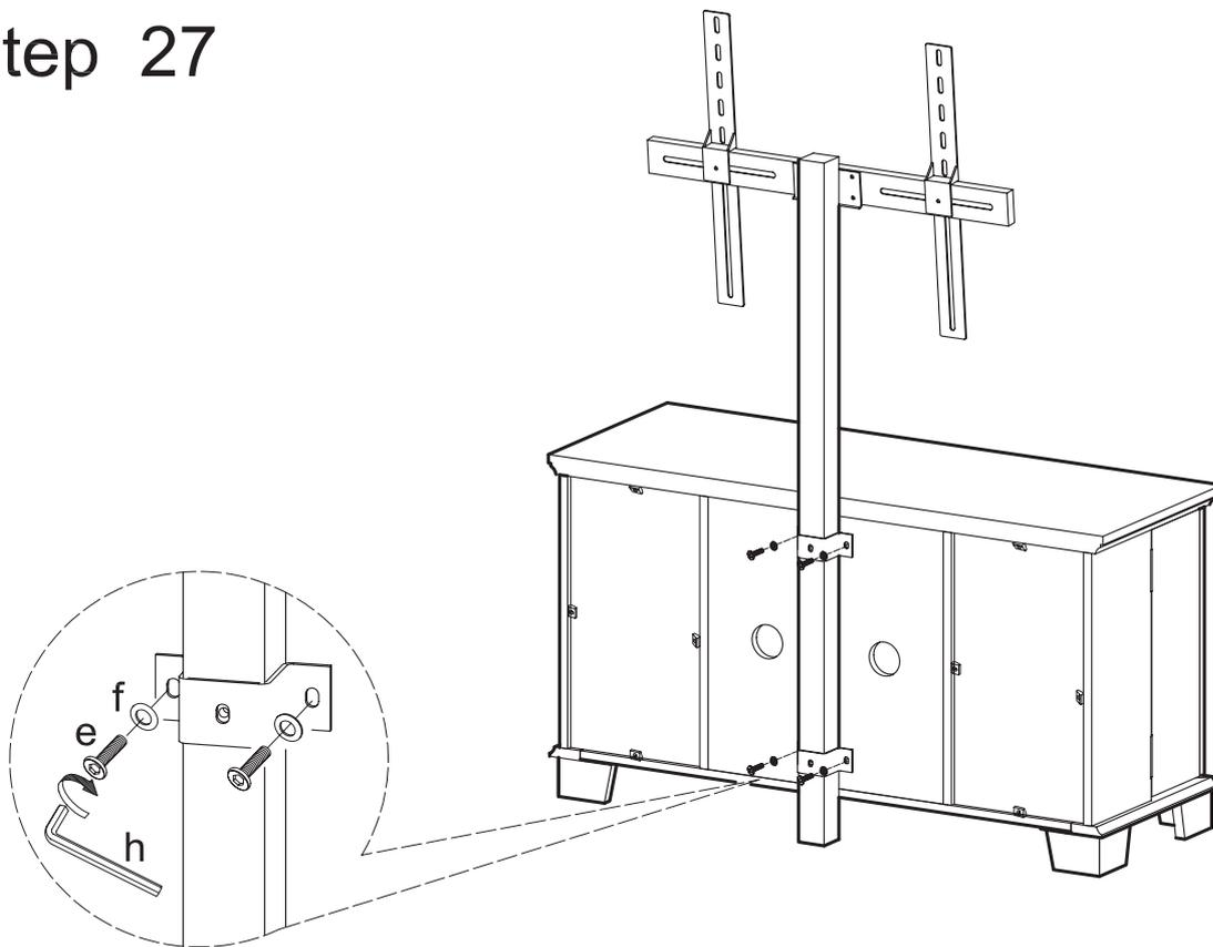
Attach TV mount to stand assembly using bolts (e) and washers (f). Tighten bolts (e) with wrench (h).
