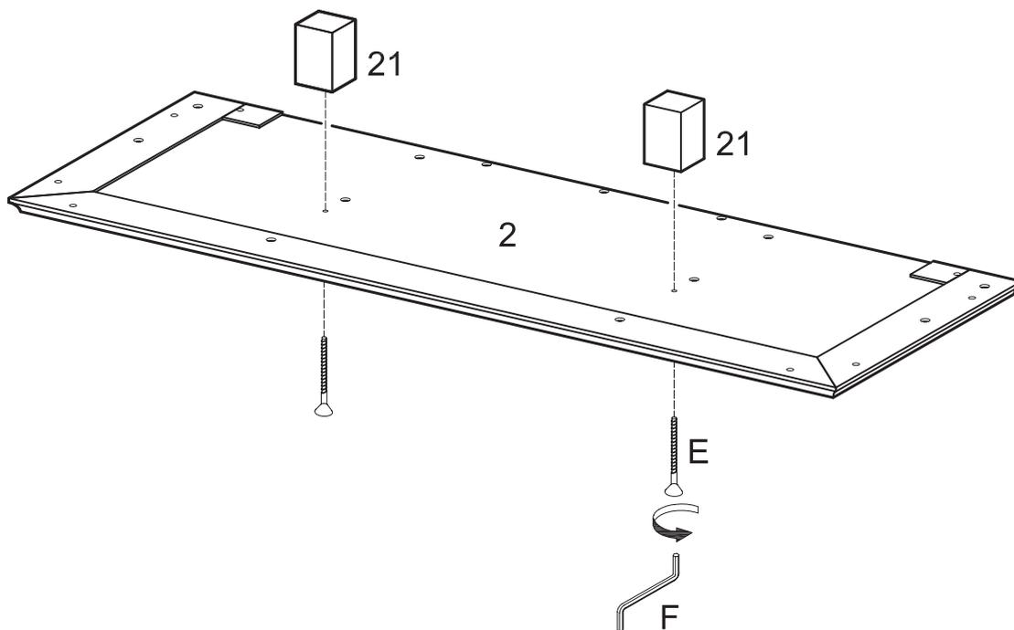
Attach stand supports (21) to stand base (2) using bolts (E). Tighten bolts (E) with wrench (F).
