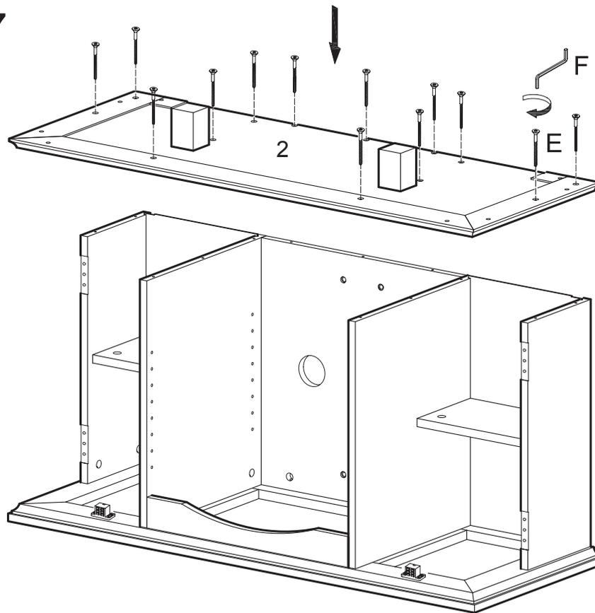
Attach stand base (2) to the stand assembly using bolts (E). Tighten bolts (E) with wrench (F).
