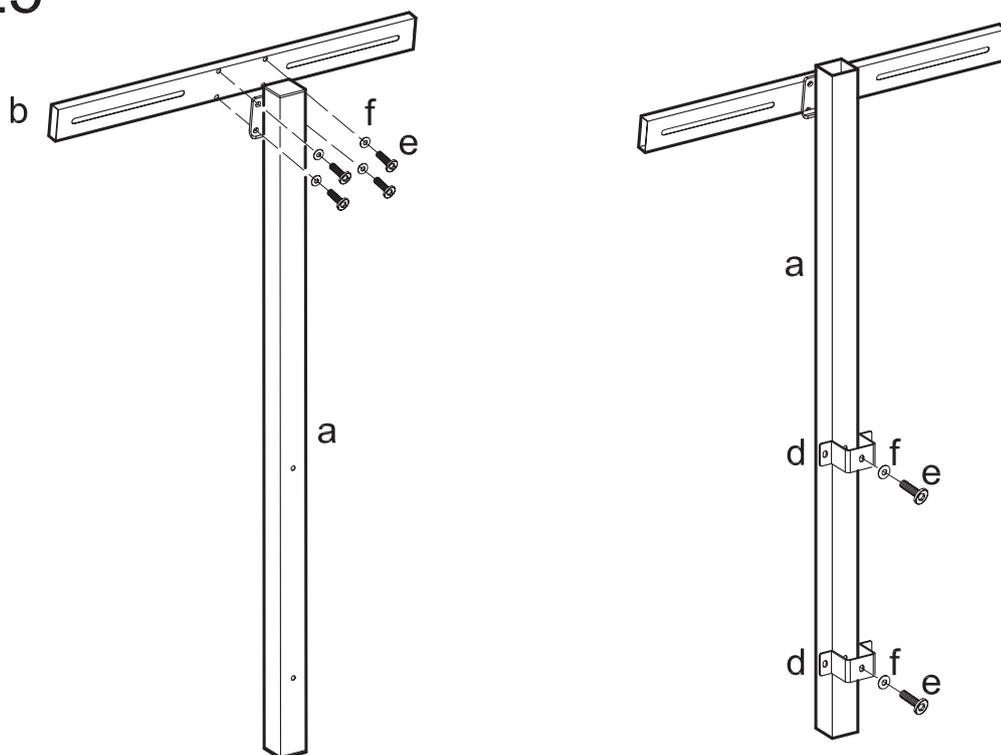
Attach lateral support bar (b) to upright support bar (a) using bolts (e) and washers (f). Attach support brackets (d) to upright support bar (a) using bolts (e) and washers (f).
