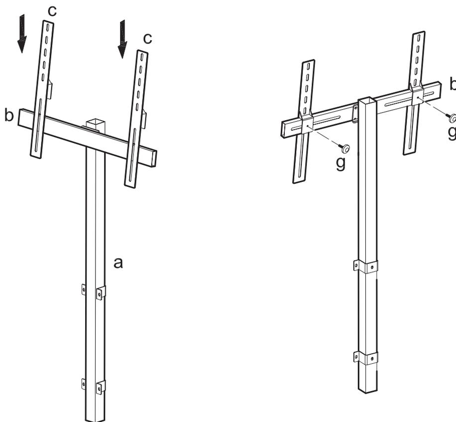
Slide mounting bars (c) onto lateral support bar (b). Secure mounting bars (c) by screwing adjustment knobs (g) into place.
