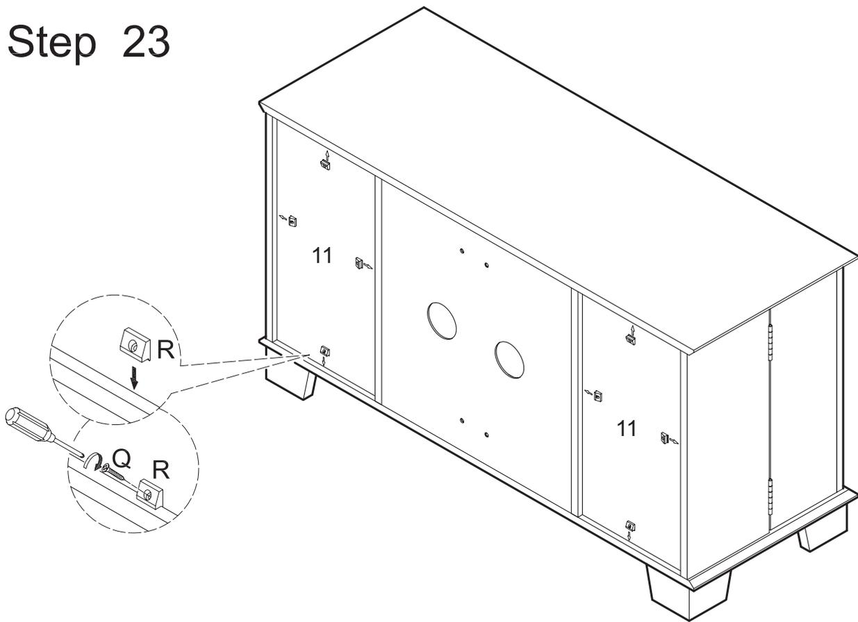
Secure back panels (11) using plastic wedges (R) and medium screws (Q).
