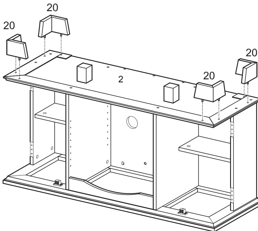
Attach feet (20) to stand base (2) using dowels as guides.
