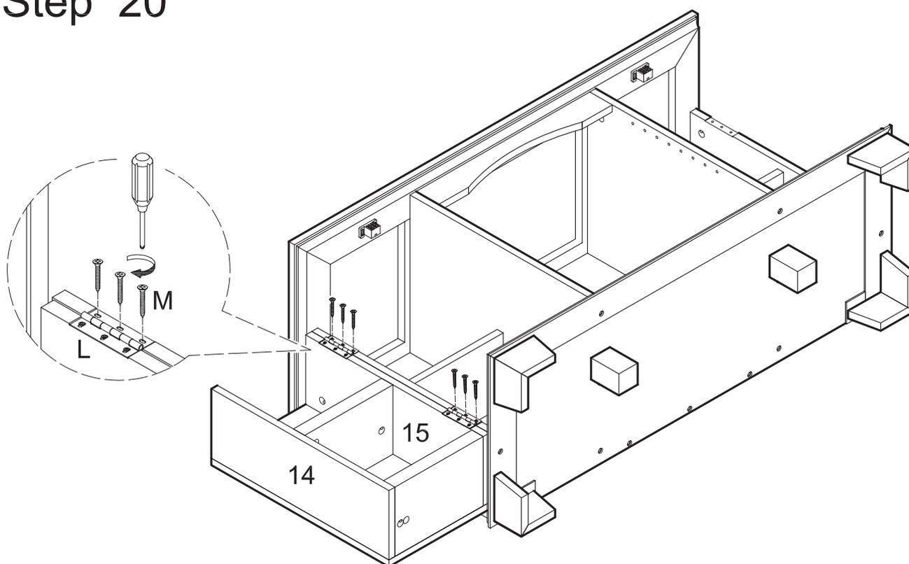
Attach door assembly (14,15) to the stand assembly at door hinges (L) using large screws (M).
