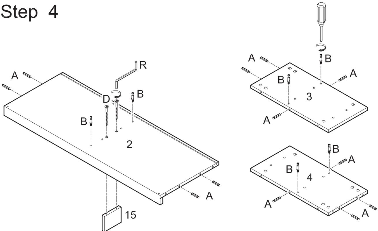
Attach support leg (15) to panel (2) using long bolts (D). Tighten long bolts (D) with wrench (R). Screw cam bolts (B) into panels (2,3,4). Insert dowels (A) into panels (2,3,4).
