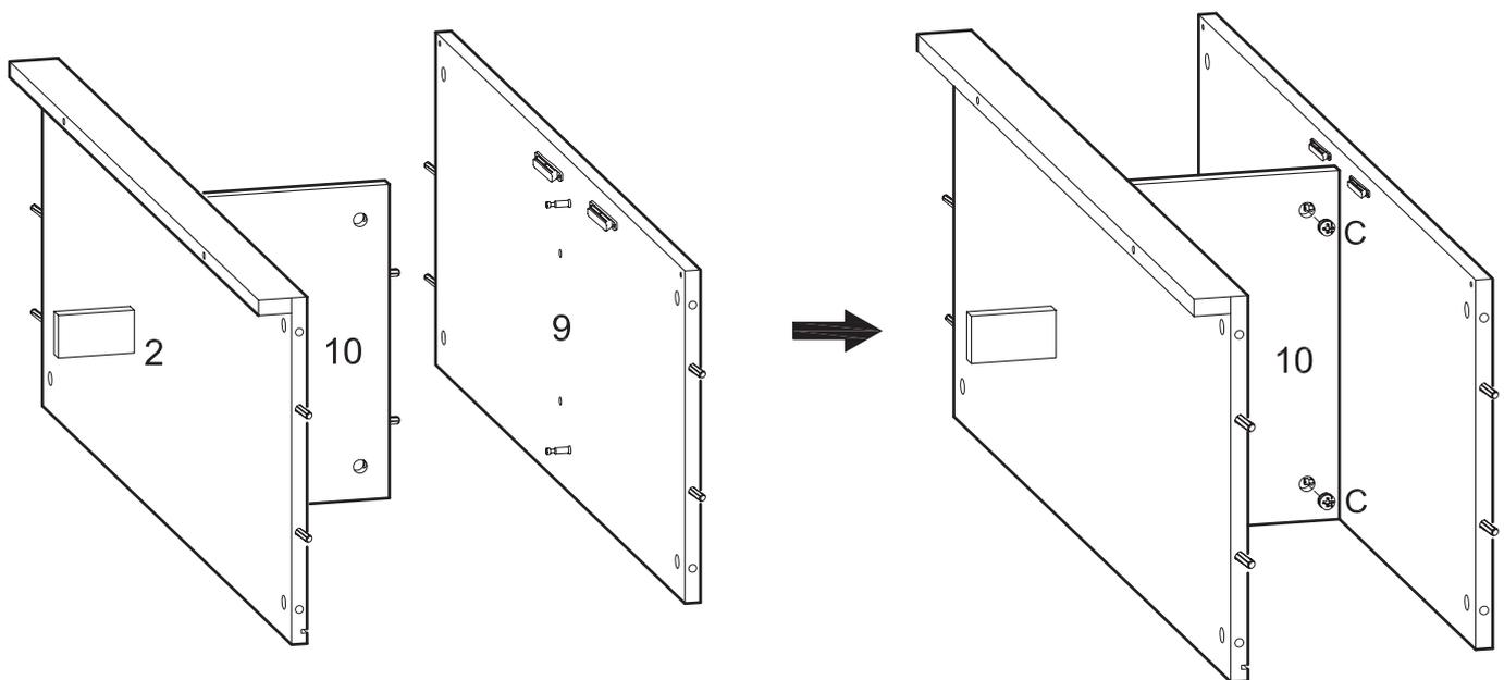
Attach shelf (9) to panel (10) using cam bolts and dowels as guides. Insert cam locks (C) into panel (10) and tighten with a screwdriver.
