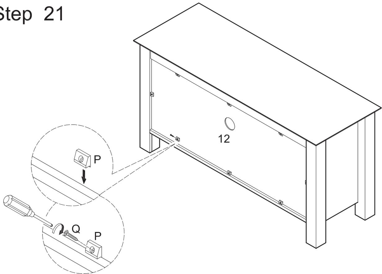
Secure back panel (12) to the frame assembly using plastic wedges (P) and large screws (Q).
