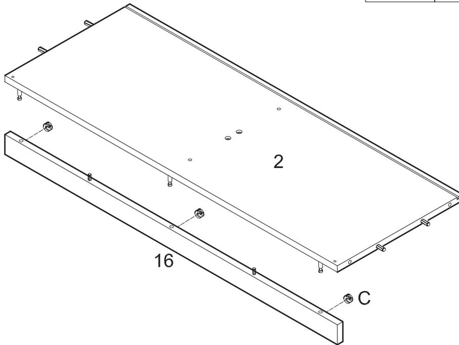
Attach slat (16) to panel (2) using cam bolts and dowels as guides. Insert cam locks (C) into slat (16) and tighten with a screwdriver.
