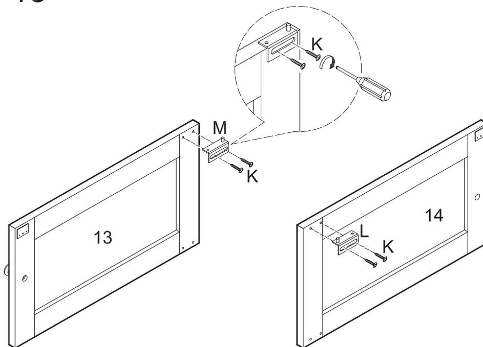
Attach door hinge (M) to door (13) using small screws (K). Attach door hinge (L) to door (14) using small screws (K).
