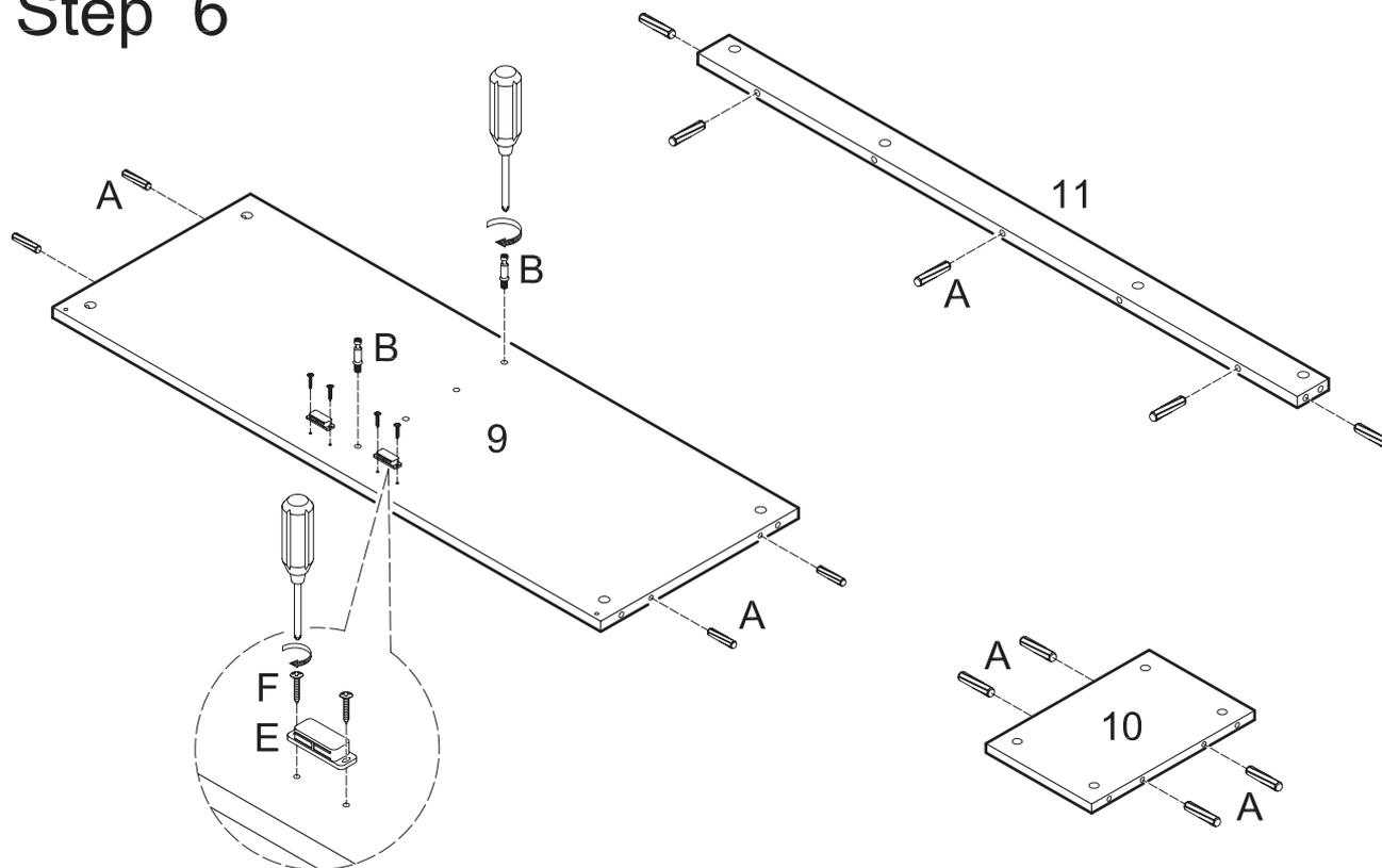
Insert dowels (A) into shelf (9), panel (10) and slat (11). Screw cam bolts (B) into shelf (9). Attach door stoppers (E) to shelf (9) using medium screws (F).
