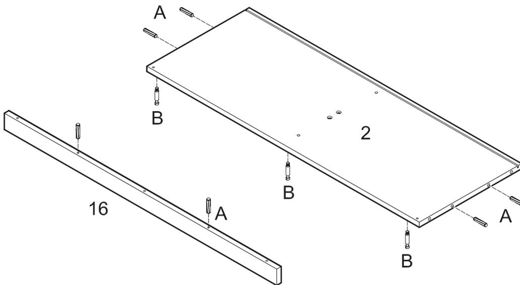
Screw cam bolts (B) into panel (2). Insert dowels (A) into panel (2) and slat (16).
