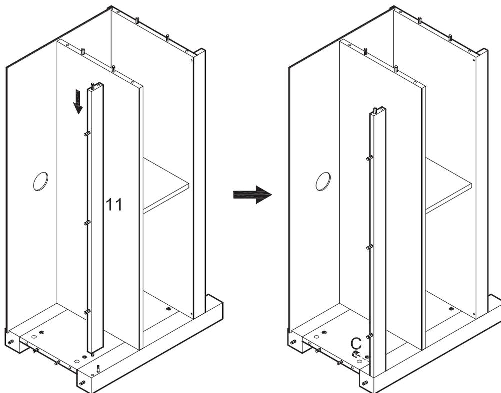
Attach slat (11) to the frame assembly using cam bolt and dowel as guides. Insert cam lock (C) into slat (11) and tighten with a screwdriver.
