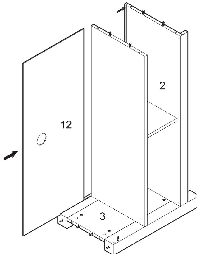
Slide back panel (12) into place. *Back panel (12) will fit into the grooves of panels (2,3).*
