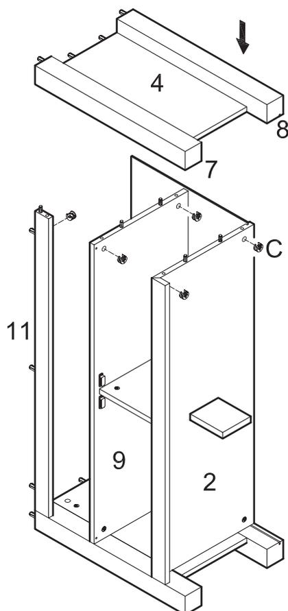
Insert cam locks (C) into panel (2), shelf (9) and slat (11). Attach the panel (4) assembly to the frame assembly using cam bolts and dowels as guides. Tighten cam locks (C) with a screwdriver.
