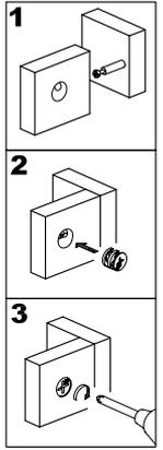
Insert cam locks (C) into the frame assembly. Attach stand top (1) to the frame assembly using cam bolts and dowels as guides. Tighten cam locks (C) with a screwdriver.
