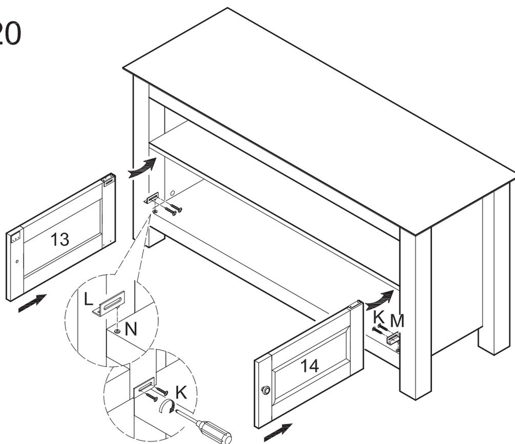
Insert door hinge (L) into left bottom plastic pivot (N). Slide door (13) into place. Attach door hinge (L) to door (13) using small screws (K). Insert door hinge (M) into right bottom plastic pivot (N). Slide door (14) into place. Attach door hinge (M) to door (14) using small screws (K).
