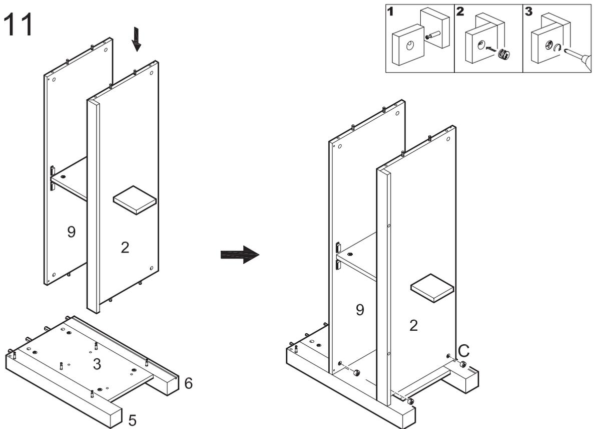
Attach the assembly from the previous step to the panel (3) assembly using cam bolts and dowels as guides. Insert cam locks (C) into panel (2) and shelf (9) and tighten with a screwdriver. *Two cam locks (C) will be inserted into panel (2) and into shelf (9).*
