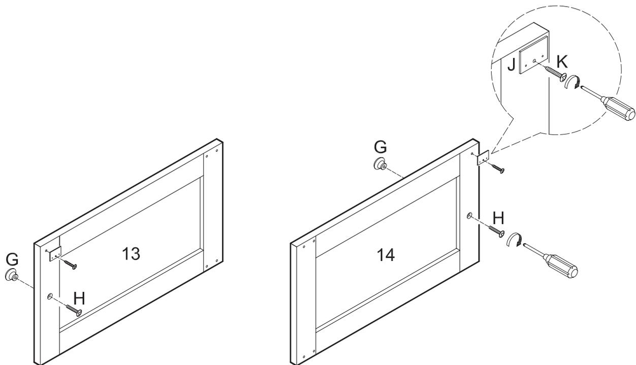
Attach handles (G) to doors (13,14) using short bolts (H). Attach door stopper plates (J) to doors (13,14) using small screws (K).
