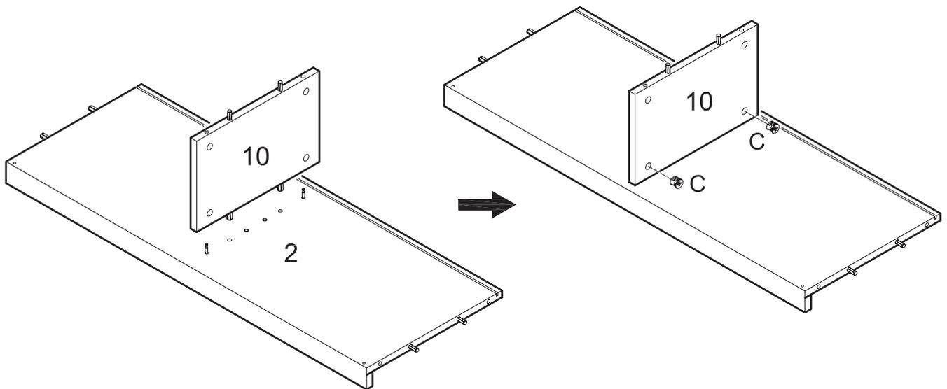
Attach panel (10) to panel (2) using cam bolts and dowels as guides. Insert cam locks (C) into panel (10) and tighten with a screwdriver.
