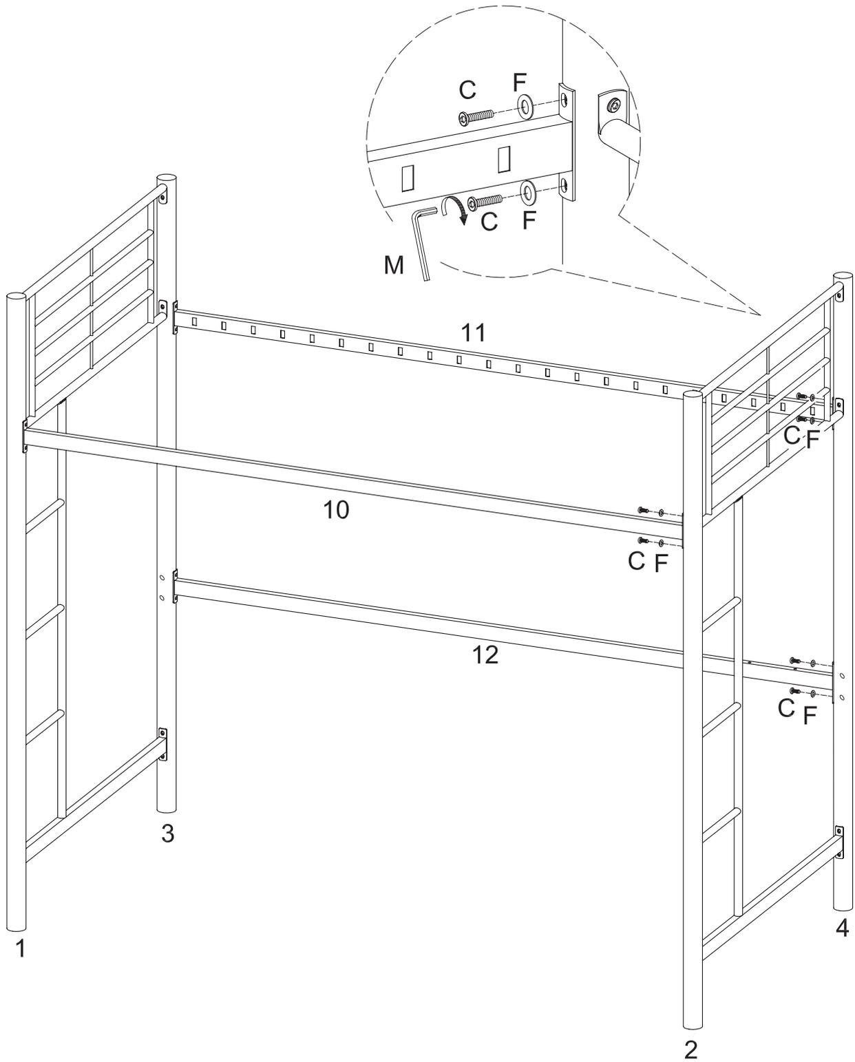
Attach crossbars (10,11,12) to the assembly from Step 6 using small bolts (C) and small washers (F). Tighten small bolts (C) with small wrench (M).
