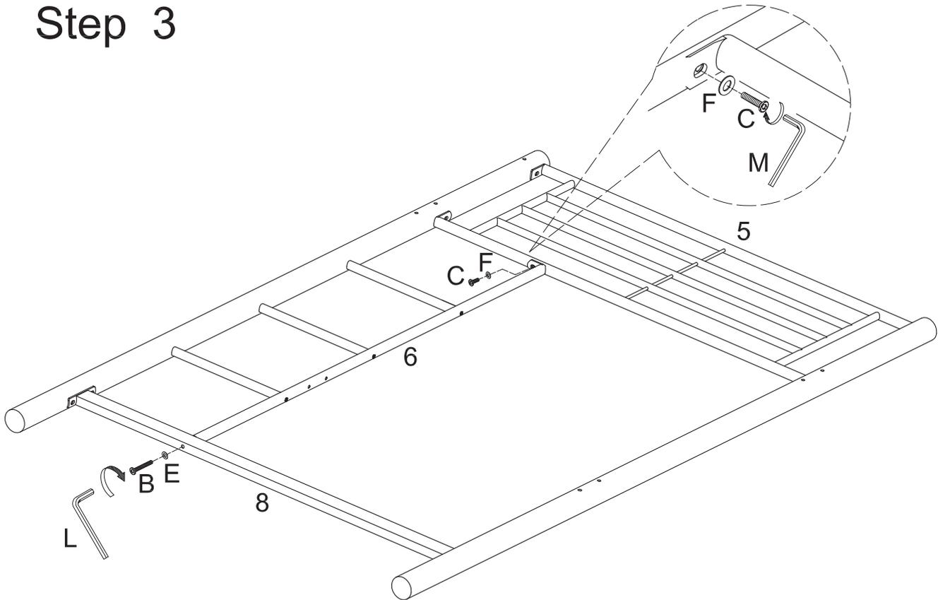
Secure ladder rail (6) to guardrail (5) using small bolt (C) and small washer (F). Secure ladder rail (6) to crossbar (8) using large bolt (B) and large washer (E). Tighten small washer (F) with small wrench (M) and large bolt (B) with large wrench (L).
