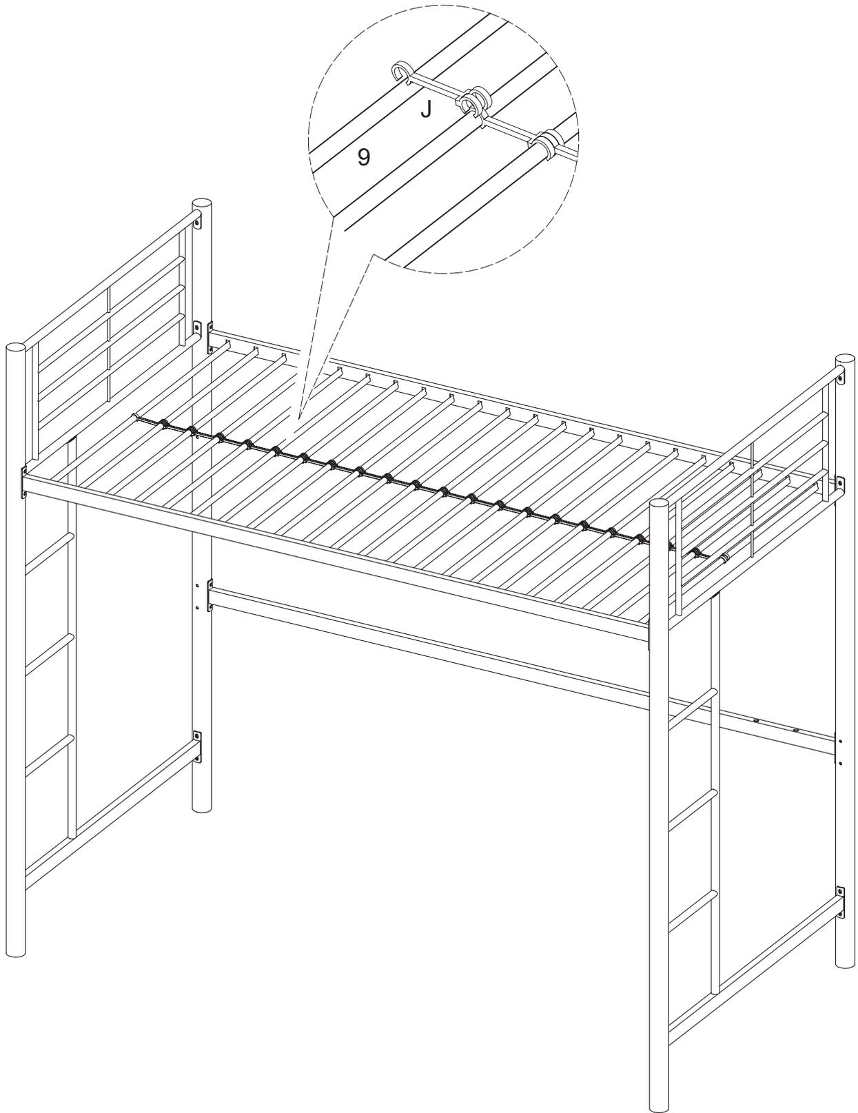
Snap plastic links (J) onto the middle of mattress support bars (9).
