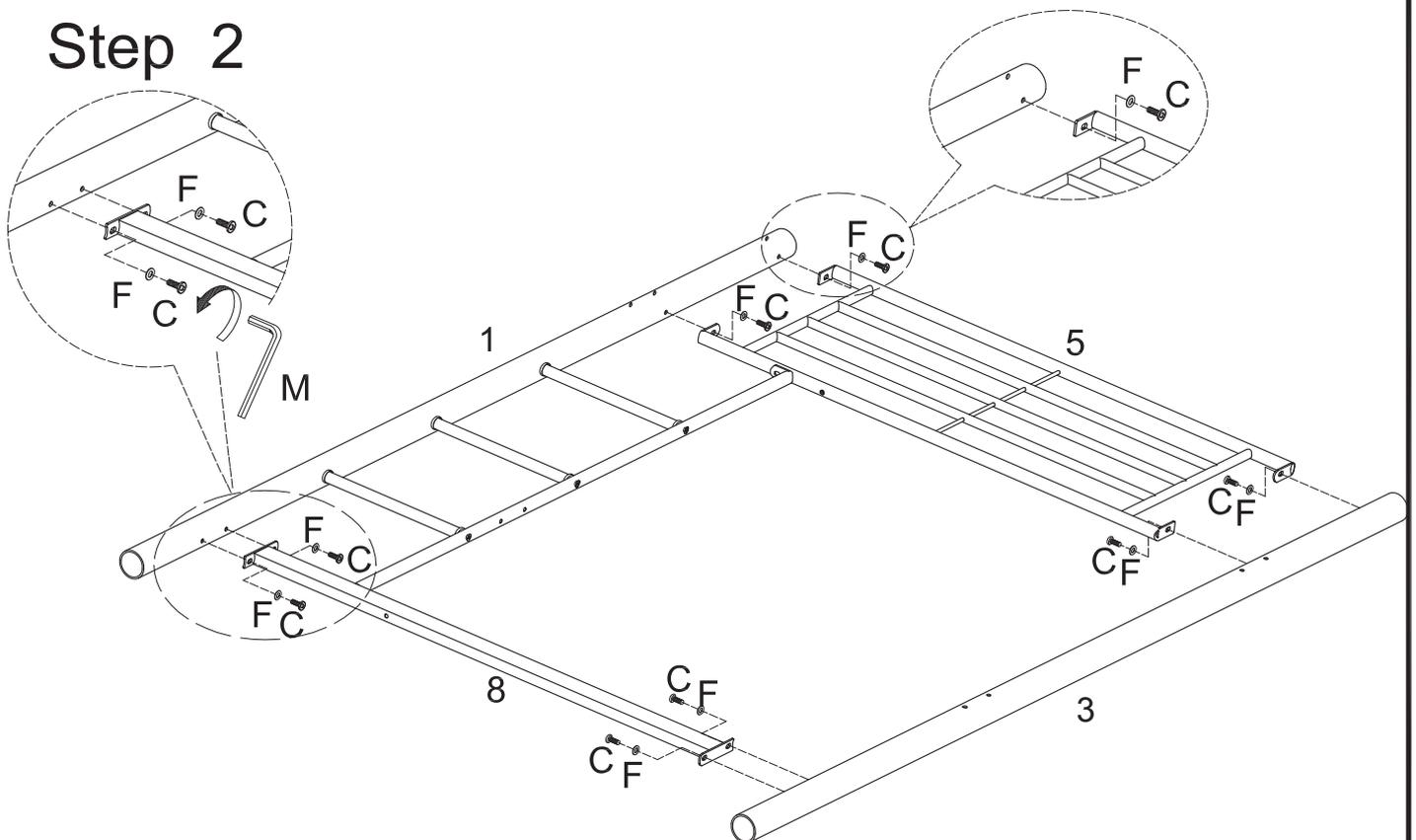
Attach guardrail (5) and crossbar (8) to post (1) using small bolts (C) and small washers (F). Attach post (3) to guardrail (5) and crossbar (8) using small bolts (C) and small washers (F). Tighten small bolts (C) with small wrench (M).
