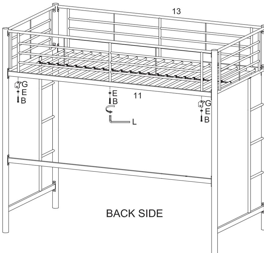
Secure front guardrail (13) to crossbar (10) using large bolts (B) and large washers (E). Secure back guardrail (13) to crossbar (11) using large bolts (B), large washers (E) and, where applicable, angle brackets (G).<sup>\*</sup> Tighten large bolts (B) with large wrench (L).
