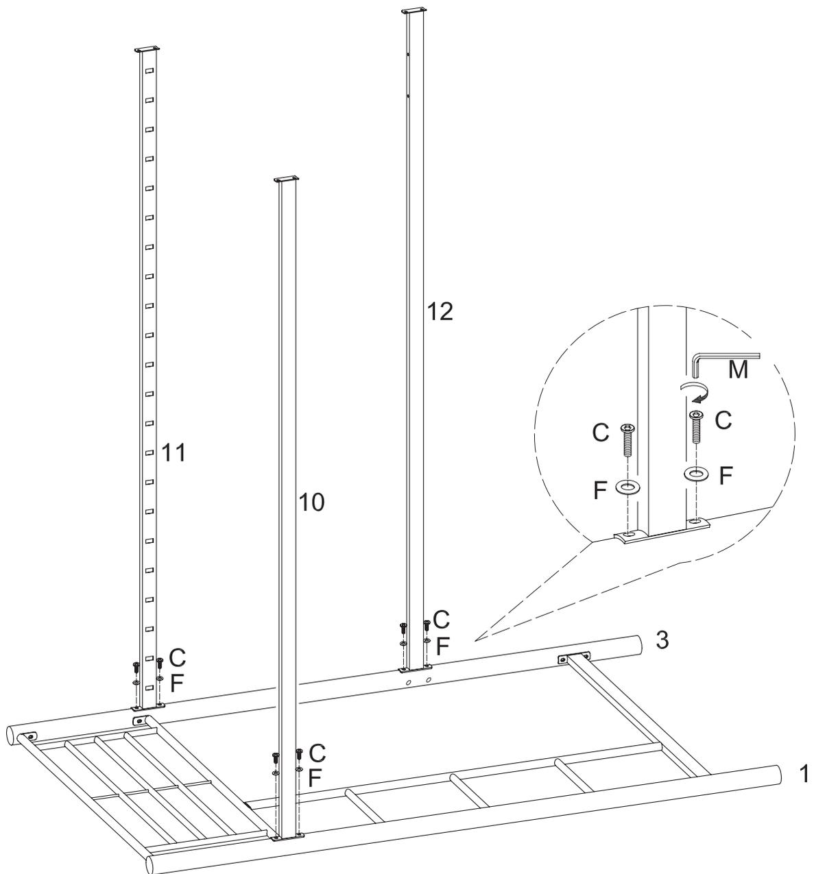
Attach crossbars (10,11,12) to the assembly from Step 3 using small bolts (C) and small washers (F). Tighten small bolts (C) with small wrench (M).
