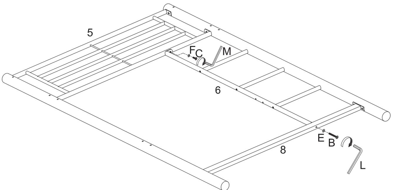
Secure ladder rail (6) to guardrail (5) using small bolt (C) and small washer (F). Secure ladder rail (6) to crossbar (8) using large bolt (B) and large washer (E). Tighten small washer (F) with small wrench (M) and large bolt (B) with large wrench (L).
