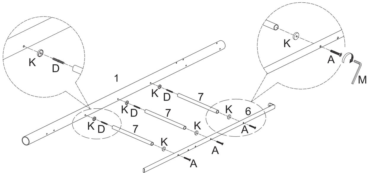
Attach post (1) to the left side of ladder rungs (7) using double-ended screws (D) and rounded washers (K). Attach ladder rail (6) to the right side of ladder rungs (7) using medium bolts (A) and rounded washers (K). Tighten medium bolts (A) with small wrench (M).
