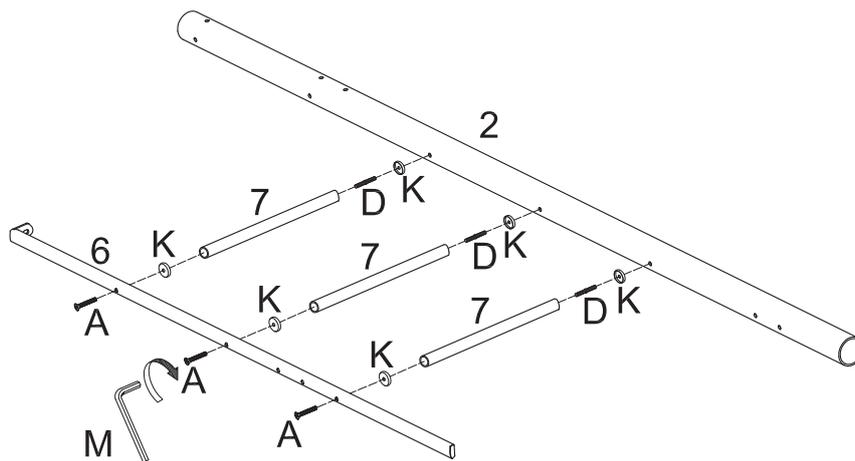
Attach post (2) to the right side of ladder rungs (7) using double-ended screws (D) and rounded washers (K). Attach ladder rail (6) to the left side of ladder rungs (7) using medium bolts (A) and rounded washers (K). Tighten medium bolts (A) with small wrench (M).
