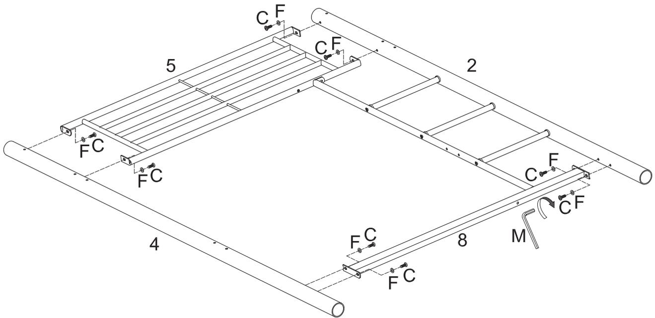
Attach guardrail (5) and crossbar (8) to post (2) using small bolts (C) and small washers (F). Attach post (4) to guardrail (5) and crossbar (8) using small bolts (C) and small washers (F). Tighten small bolts (C) with small wrench (M).
