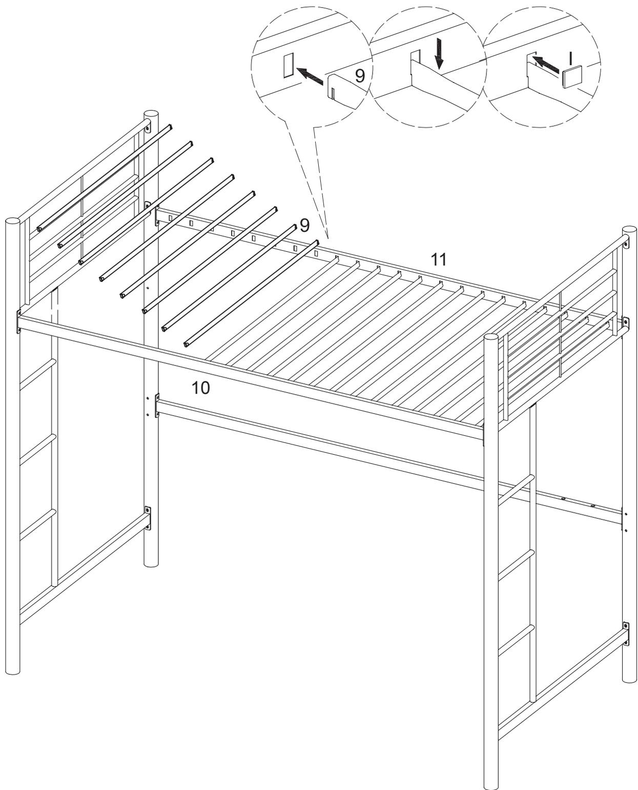
Insert mattress support bars (9) into the provided slots of crossbars (10,11). Secure mattress support bars (9) by snapping plastic tab locks (I) into the provided slots of crossbars (10,11). *Note that it may be necessary to apply more pressure to some plastic tab locks than others.*
