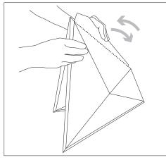
STEP 2 Carefully fold the locking tab as shown to prevent wrinkling or damage to tile.
