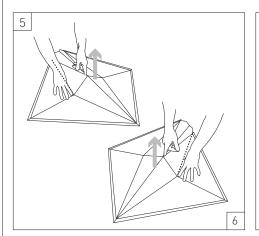
STEP 5 Hold down the tile as shown, then insert finger into center hole and lift to crease the inner folds. STEP 6 Repeat on other side.
