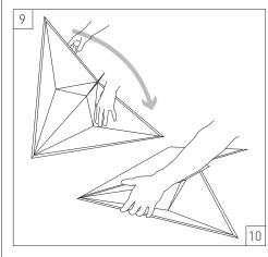
STEP 9-10 Gently start to fold tile over, making sure not to let the edges bow. Continue to fold over to release tension in the creases. This will allow the tile to sit flat in the drop ceiling grid.
