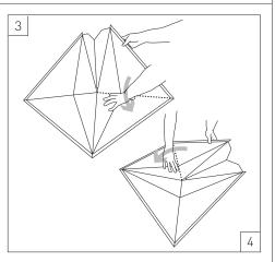
STEP 3 Carefully fold along the other axis. Do not apply excessive force or the tile will crease. STEP 4 Repeat on the other side.
