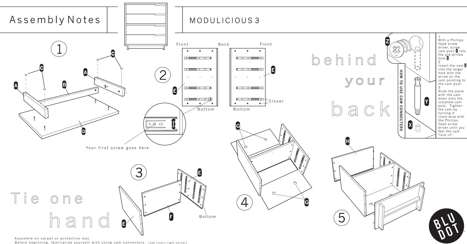
See Sketch 1. Screw the cam post into the small hole on the side of each foot 🛕 . Place the two cams in the stretcher 🖪 so that the arrow points towards the end of the stretcher and turn the cams to the right until snug.
