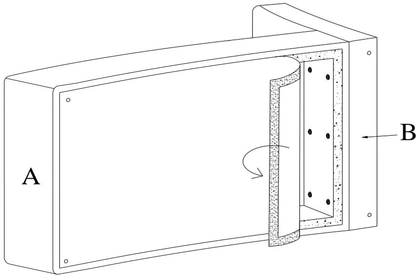
Then close Velcro Strip on the bottom of Seat (Part A) as shown.
