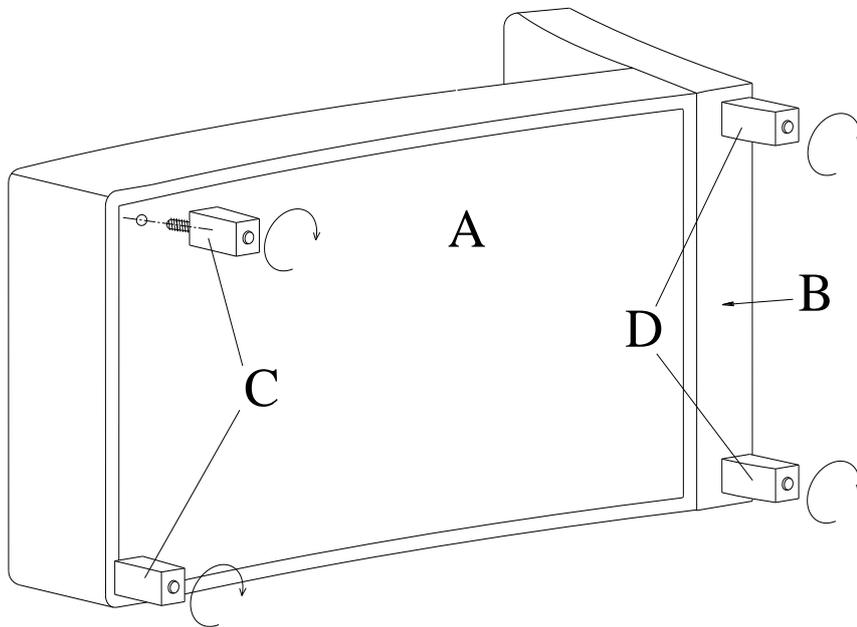
Attach Front Legs (Part C) and the Back Legs (part D) into the Seat (A)'s pre-drilled holes by hand rotating. Tighten them by hand as shown in Figure 1.
