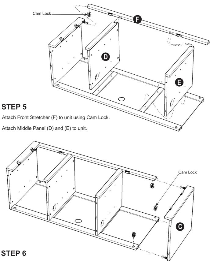
Attach Side Panel (C) to unit using Cam Locks.
