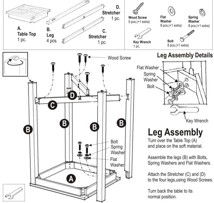
Please keep the Key Wrench as you may need to retighten the Bolts in the future. *Tools required for assembly : <u>Philips</u> screwdriver*
