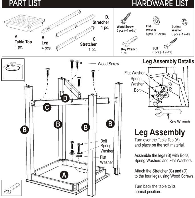
Please keep the Key Wrench as you may need to retighten the Bolts in the future. *Tools required for assembly : <u>Philips</u> screwdriver*
