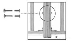
When the two Gate pieces are placed together, the inner posts are longer at the bottom of the Gate
