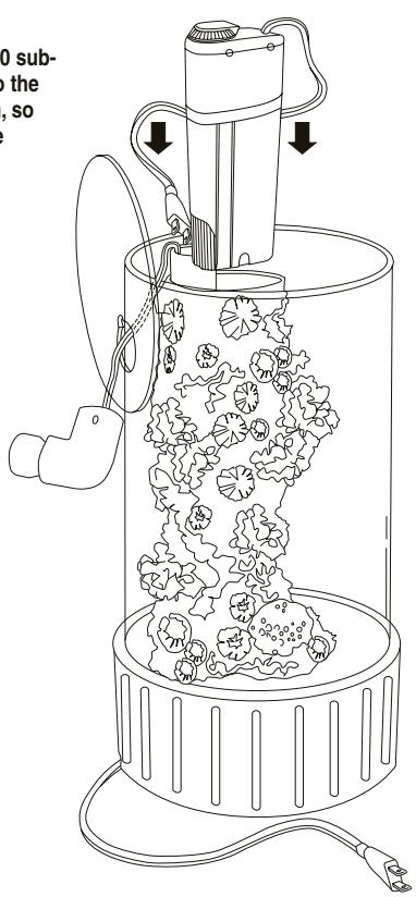
**5** Insert the Duetto 100 submersible power filter into the reef sculpture, as shown, so that the section cups are against the dry tube.
