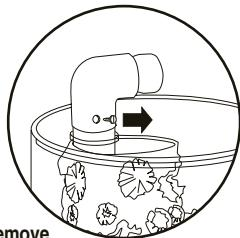
**2** Remove screw from base of light fixture.
