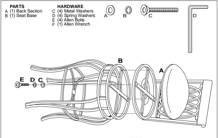
NOTE: ASSEMBLY DRAWING IS OF A GENERIC STOOL. THE SEAT CUSHION SHOULD BE PRE-ATTACHED, BUT NOT DRAWN HERE TO SHOW THE ASSEMBLY OF THE STOOL.
