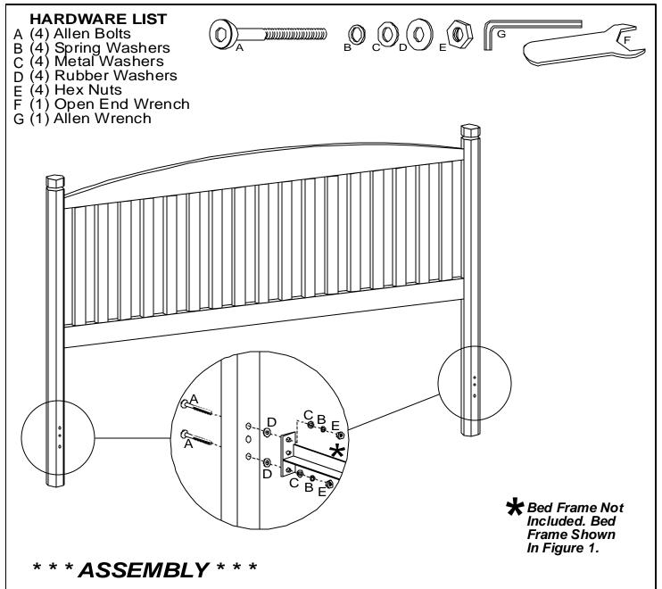
Attach each Bed Frame (\*Not Included) to posts on Headboard, using 2 Allen Bolts (A), 2 Rubber Washers (D), 2 Metal Washers (C), 2 Spring Washers (B) & 2 Hex Nuts (E) per each side. Only Hand Tighten Bolts & Nuts using Allen Wrench & Open End Wrench (G & F) once both bed frames have been attached. See Figure above for illustrated details.
