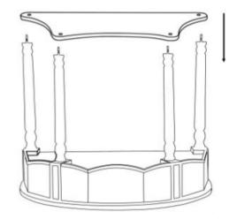
Lay out all parts listed above on soft, clean and dry suface. Install legs by tightening screws to table top. Color lables should match up on legs and table top. Please note that screws should not be fully tightened at this step.
