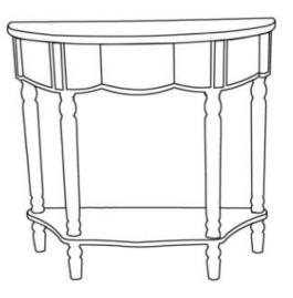
If the table isn't on same level, adjust leg levelers on bottom of legs a bit.
