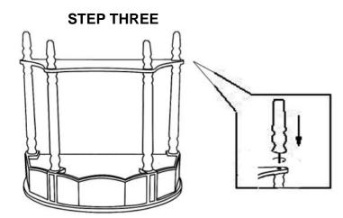
Install extension legs and screw up all parts below table top, then turn the adjustable hardware.
