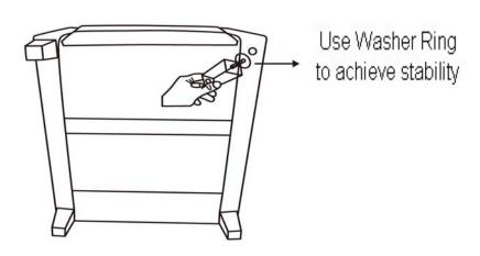
Install the first leg into the bottom of the chair by placing 1 plastic washer ring (improvees tightness and security of leg) onto the threaded stem.
