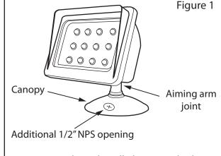
For a rain-tight seal, caulk the top and sides of the canopy and the aiming arm joint(s).
