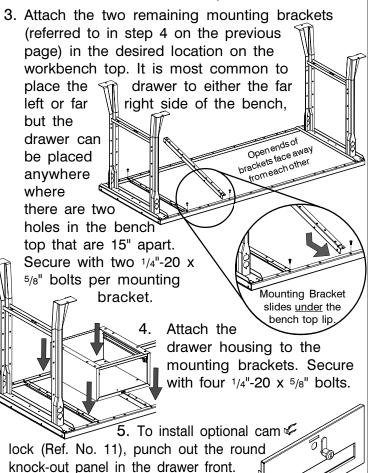
lock (Ref. No. 11), punch out the round knock-out panel in the drawer front. Then insert the cam lock through the hole, and secure with forked clip.
