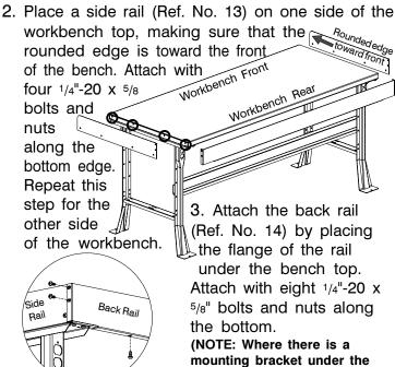
4. Attach the back rail to the side rails, using two 1/4"-20 x 5/8" bolts and nuts on each end.
