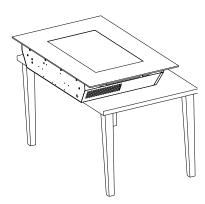
• Attach the floor standing base to the fireplace using the provided screws.
