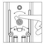
Switch the Cam position to R if the door is right-sided and vice versa. Caution: Be sure the cam is turned to the correct
