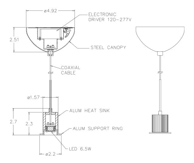
CONSTRUCTION: 59" coaxial cable suspension for flexible mounting heights
