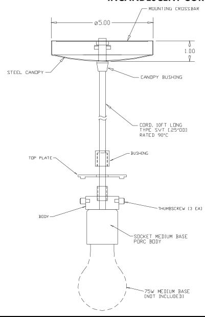
**CONSTRUCTION:** 10' clear cord suspension for flexible mounting heights
