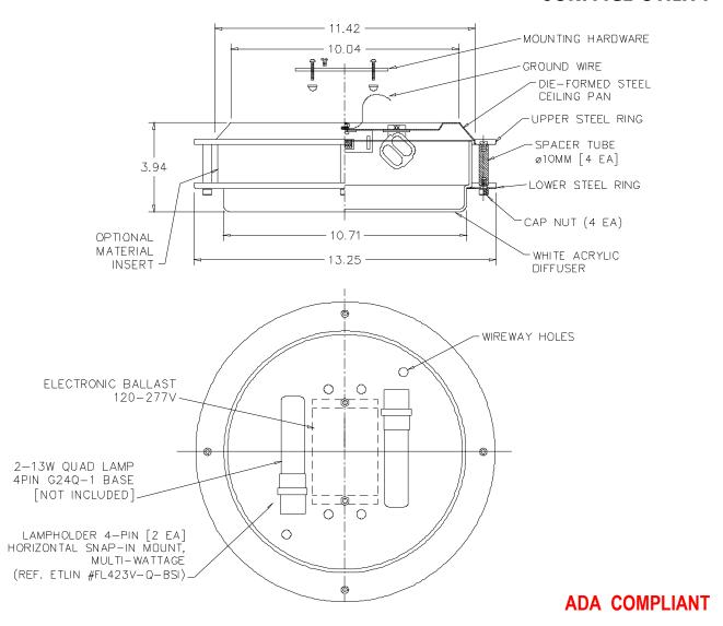
CONSTRUCTION: Steel Pan, Etched White Acrylic diffuser
