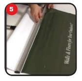
Slide the graphic between the hinged edge and the rail through the narrow opening. Snap shut to secure.
