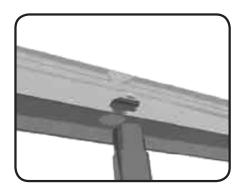
Position the hole in the rail over the pole.
