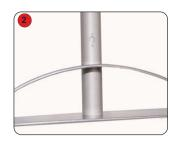
Align mounting holes to face the flat sides of the feet.
