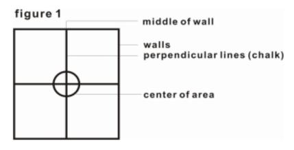
Start from the center of the room ensuring that the tile is laid exactly along the chalk lines. The tiles easily connect like puzzle pieces together.
